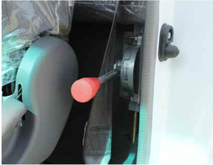
The Joystick at UPPER place The Aerial Platform Truck can work .
